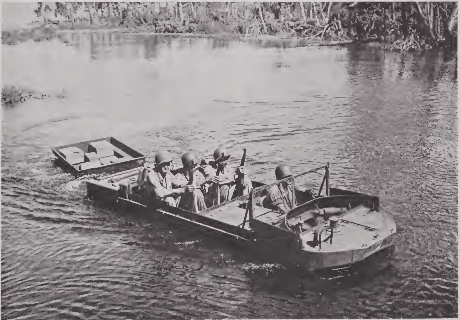
FIGURE 75. M-29C Weasel with amphibious trailer gets through deep water in Solomon Islands.
